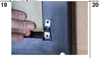
The spring must rest on the plate!
