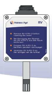
The RV-sensor measures the relative air humidity in a room and converts it into an electrical signal. This signal can be used, by means of a climate computer (ORION or SIRIUS), to guard the humidity. If necessary, the climate computer can control a humidifying unit and / or adapt the ventilation.
