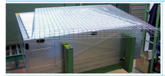
Put the pyramidal shape mesh (ref.8.5/Optional kits) on the fan as in the picture. The rectangular holes must be positioned horizontally.
