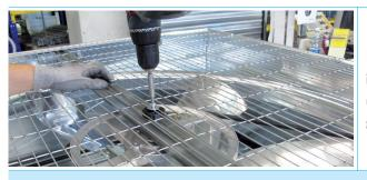
Fix the screw with the washer (ref.7.13/Bolts&nuts) into the central pulley axle. Fix all the components by using the pneumatic screwdriver (ref.3/Assembling tools).
