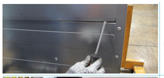
By means of a screwdriver (ref.13/Assembling tools) insert cover plate (ref.1.3/Body) over the fan housing.
